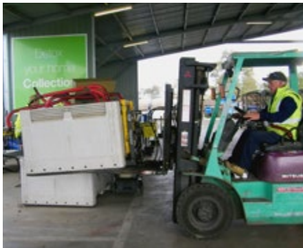
Forklift with lifter
